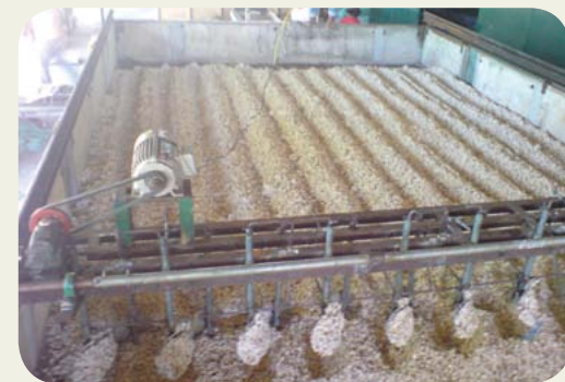
Prototype mixer for drying granulated cassava in flatbed dryer.
