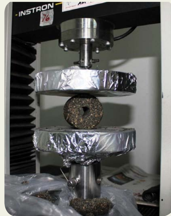
Laboratory testing of different carbonized rice hull briquette formulations
